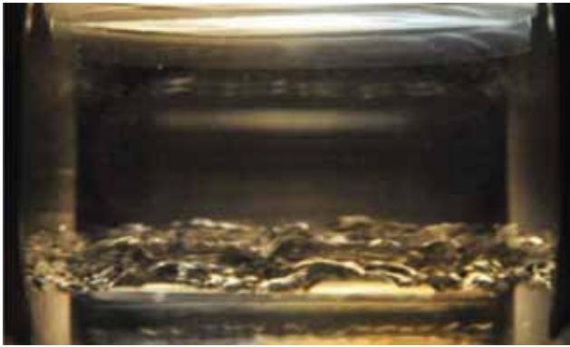
Steam and condensate flow
