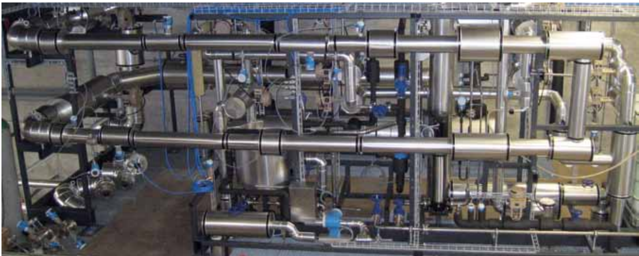
Meet ALICE, a rig built to study steam measurement
